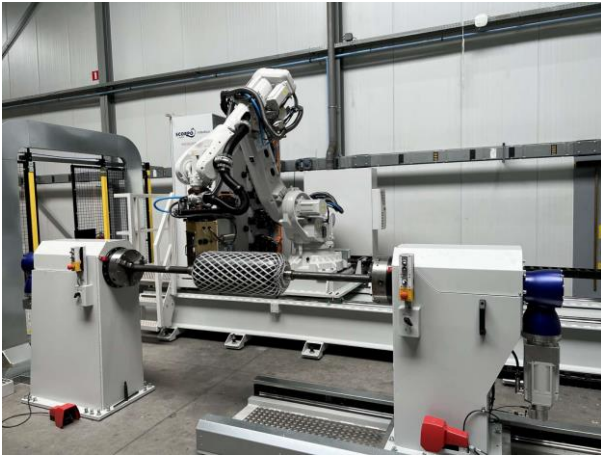
TANIQ robotic winding system for GKN Fokker
